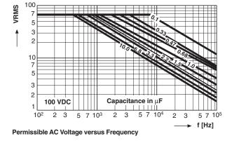
Permissible AC Voltage versus Frequency
